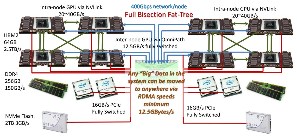
~2.3 Terabytes/node Hierarchical Memory for Big Data / AI (c.f. K-computer 16GB/node)
